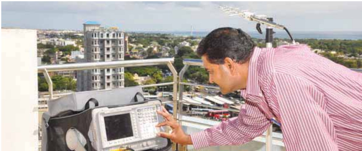
In-situ measurement using Spectrum Analyzer
