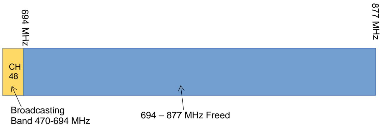
Figure 2: 700 MHz and 800 MHz Spectral Occupancy after 30 June 2019
