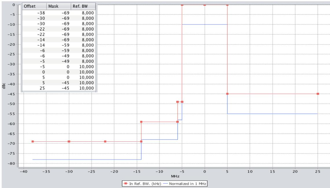
**Figure B8:** LTE800 Downlink Emission mask
