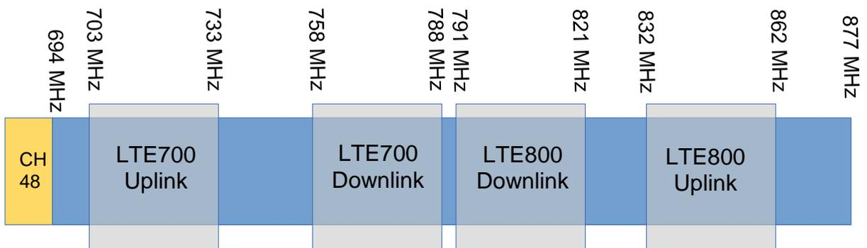
Figure 3: 700 MHz and 800 MHz Band Plans
