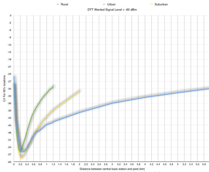
**Figure B10: C/I vs distance for C=-60 dBm**
