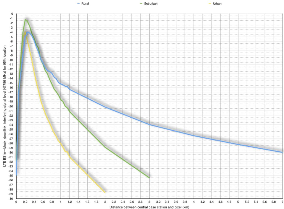
**Figure B9:** In-block IRSS against distance
