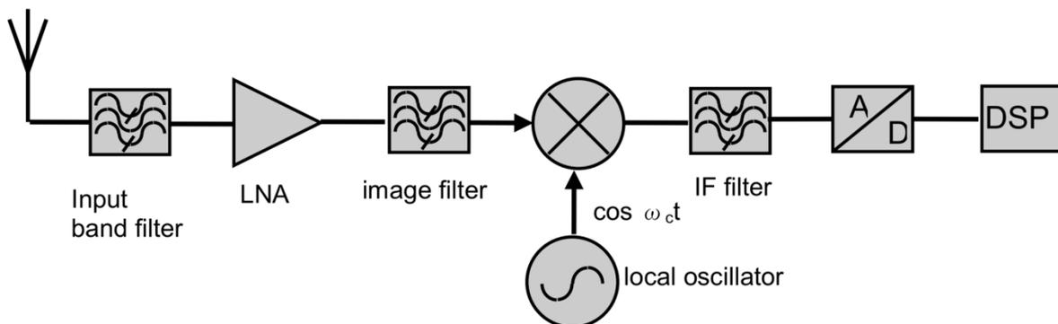
**Figure B4:** Front-end of superheterodyne Receiver
