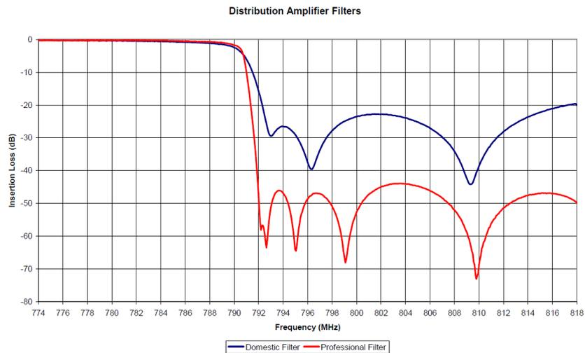
**Figure B6:** Distribution Amplifier Filters considered in coexistence study (Source: ERA Technologies<sup>21</sup>)
