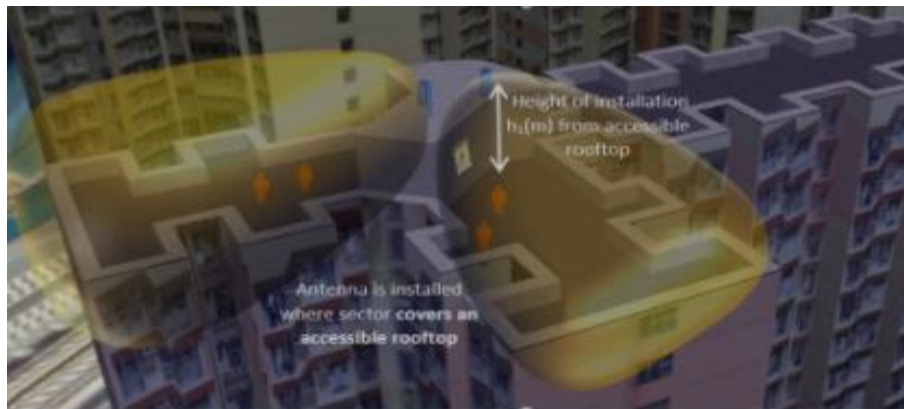
Figure 13 Antenna propagation covers an accessible rooftop
