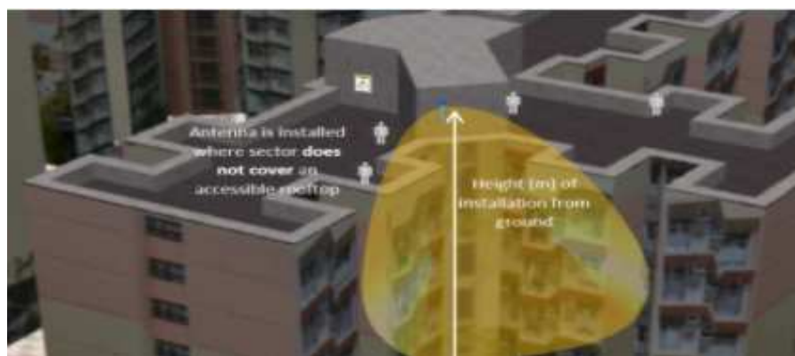
Figure 8. Installation of antenna from ground to centre of radiation
